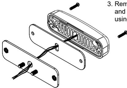
3. Remove the outer housing of the Versa Star<sup>®</sup> light and attach the light to the BB274-FISUV-VER bracket using the screws that came with the light.
