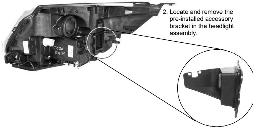
2. Locate and remove the pre-installed accessory bracket in the headlight assembly.
